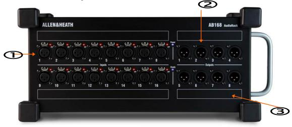
**Input sockets** 16 balanced XLR nite inputs with +48V Phantom Power indicator. The preamps are built into the AB168 and their Gain, Pad and 48V phantom power are remote controlled from the mixer via the dSNAKE link. The outputs of the analogue preamps are converted to digital format and transported via dSNAKE to be processed and mixed at the GLD or Qu mixer.
