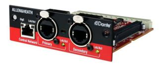
M-Dante is one of a range of digital audio networking options available for dLive, GLD and iLive to enable integration with other systems, digital mic splitting, multi-track recording and system expansion. It provides 64 channels of bi-directional audio at 48kHz, and can be fitted to any dLive I/O Port when equipped with a M-DL-ADAPT interface.
