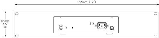
The **MPS12** is supplied ready for rack mounting. For free standing use, remove the 19" front panel, which is secured by four M4x8 Pozi screws and shakeproof washers.
