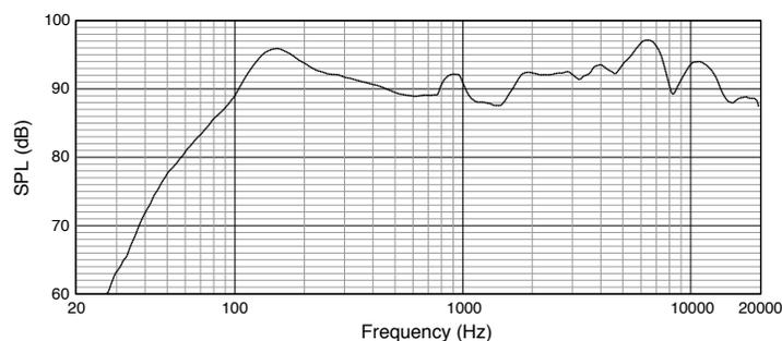
Frequency response chart (2pi, mounted in ceiling), 100V input on 30W tap, measured at 4 meters
