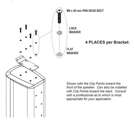
**Step 3:** Suspend the attached suspension bracket system via the 15 mm (0.62 in) Clip Points located on the 30 degree bend on each bracket. Be sure to consult the building codes in your area to determine the proper materials and procedures.
