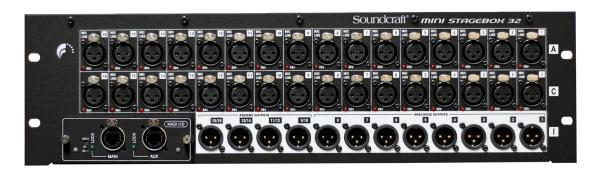
The Mini Stagebox 32R (3U) provides 32 analogue inputs and 8 analogue line outputs, with 4 pairs of AES outputs, providing a total I/O capacity of 32 inputs and 16 outputs, with the Mini Stagebox 16R (2U) model providing 16 analogue inputs and 8 line outputs making a 16 x 8 matrix.
