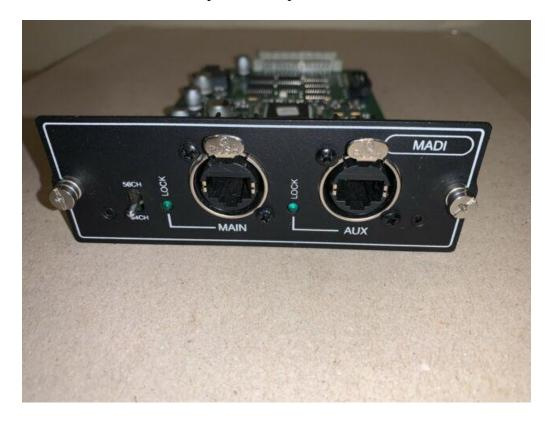
The MADI I/O card can establish a 64-channel MADI input and output to a remote device such as stage rack, another console or Broadcast feed to an OB. Optical inputs and outputs are provided on SC connectors available in multi-mode versions only. The auxiliary interface can be used as a redundant link. A Cat5 version of the card is also available. A toggle switch allows the card to be switched from 64ch to 56ch mode for compatibility with older MADI devices.
