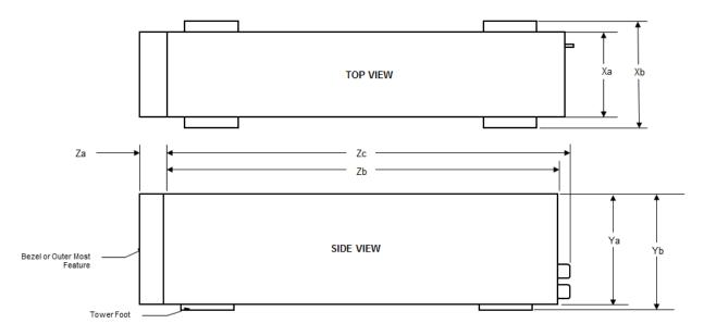
Figure 3. Chassis dimensions
