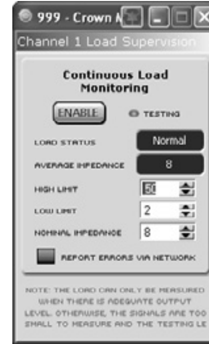
Figure 4.6 MA-i Load Monitoring Panel
