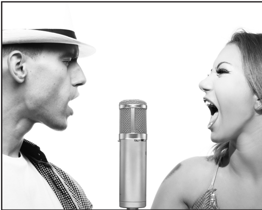
In this image, two vocalist perform at the same time on either side of the WA-47jr using a figure-of-eight pattern.
