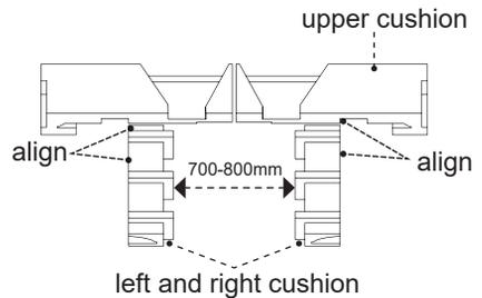
2. Two people stand on each side of the television. Hold the back side of TV with one hand and grasp the buckle on lower box with the other hand. Place the TV on the cushions with the screen face upward. Make the handle touch upper cushion, back cover touch the left and right cushions. When finished, take off the lower box.
