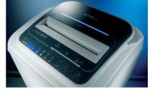
**Touch Screen Panel** Just touch the controls to activate the machine functions. Keep your finger on the "Forward" control for 5 seconds and the machine functions continuously for 30 seconds when transparent material needs to be shredded. A visual signal notifies the operator when the blades should be lubricated for improved cutting capacity.
