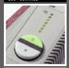
"ECC" - Electronic Capacity Control indicates the used sheet capacity during shredding process to avoid paper jams.
