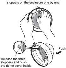
Bend the enclosure to release the three
