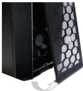
Easy fan installation without removing the full front bezel, but simply by removing the front panel
