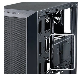
SSD can also be installed behind the motherboard tray
