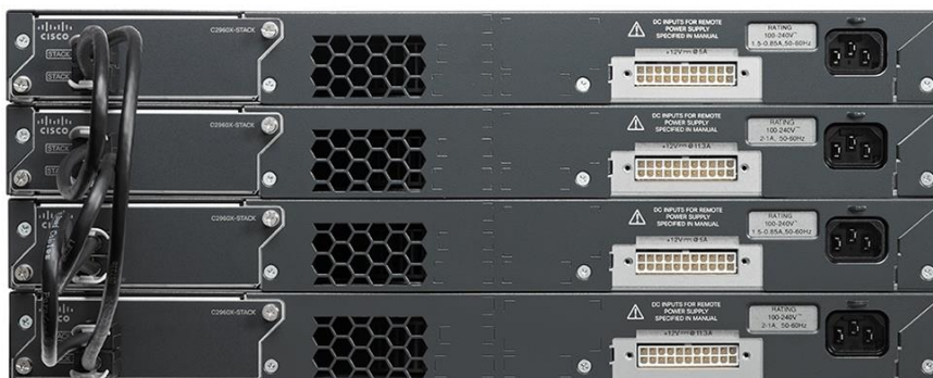
Figure 2. Cisco FlexStack-Plus Switch Stack
