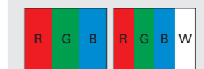
RGB alignment RGBW alignment RGBW alignment with enhanced brightness achieved by employing more white dots
